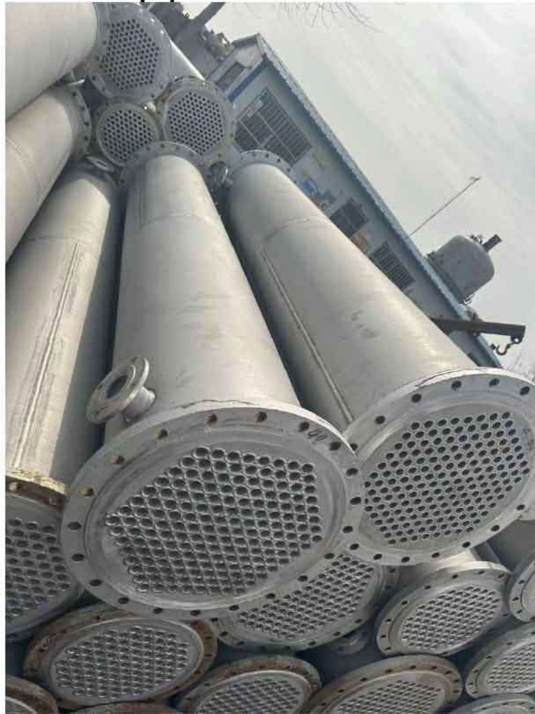
3.Photo of Condenser:40m2 equip with 20m3 reactor
